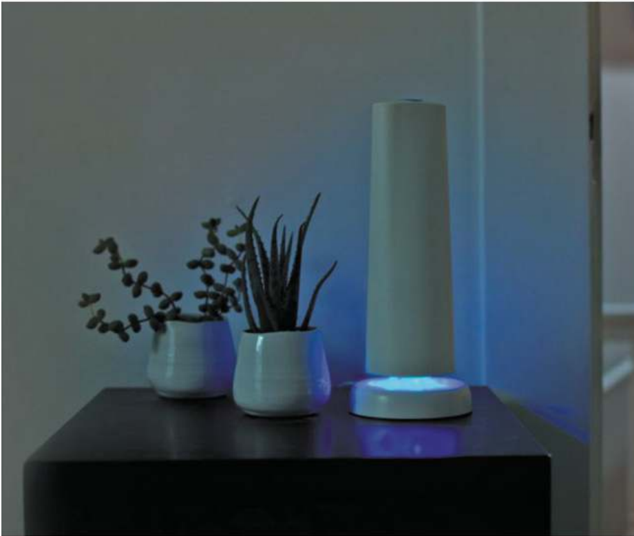
The base station's blue light turns off upon an alarm to make it difficult for an intruder to find it. But the sound of the system's onboard siren still comes from its base station, making it easily identifiable.
