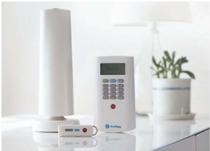
Forensic alarm and security expert Jeff Zwirn (top) puts a SimpliSafe system through its paces. The system consists of base station, keypad, several types of sensors/detectors, door contacts, wireless siren (in addition to the base station's built-in siren) and a wireless panic button and/or key-chain remote.
